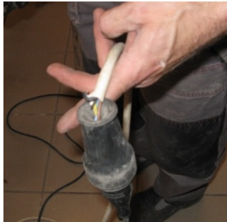
Damaged extension leads
