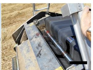
An employee climbed up on a round baler that was in operation. The baler was attached to a tractor by a rubber band. His right arm was caught in the top shaft of the machine on which the rubber band was running, and was ripped from his body.
